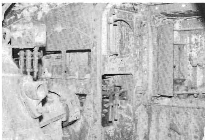
The inside of the Mk. IV was cramped and difficult to work in. This angle illustrates how close the gearsman and the gunner at the rear sponson position were to each other. The transmission is on the left of the photo.
